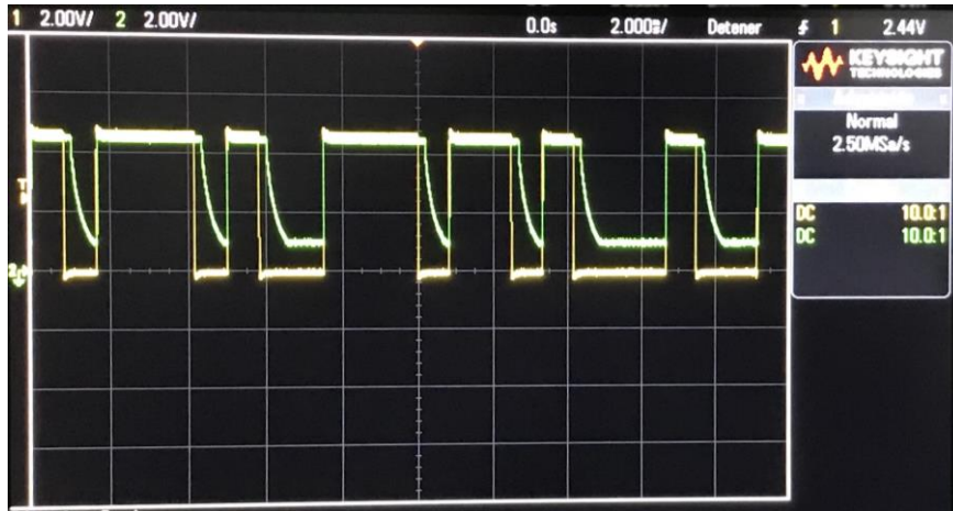
Figure 3-9 Case 1 oscilloscope display. The yellow signal is measured at the transmitter signal and the green one at the receiver.
