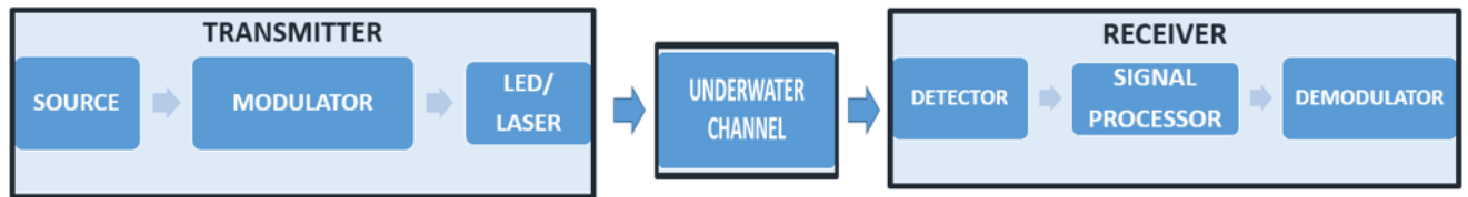
Figure 2-2 Simplified example of Optical communication [15].
