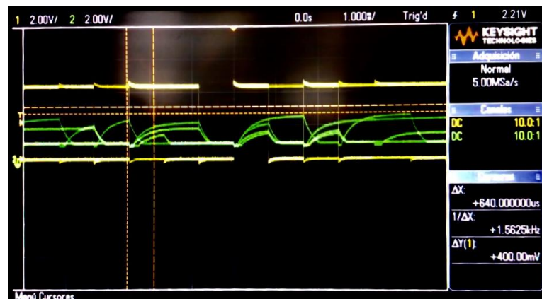
Figure 3-30 Capture of an oscilloscope display video in which the water in the tank was turbulent. It can be seen how the received signal is fluctuating and unstable.
