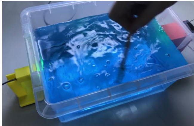
Figure 3-16 Water tank with turbulence affects UOWC.
