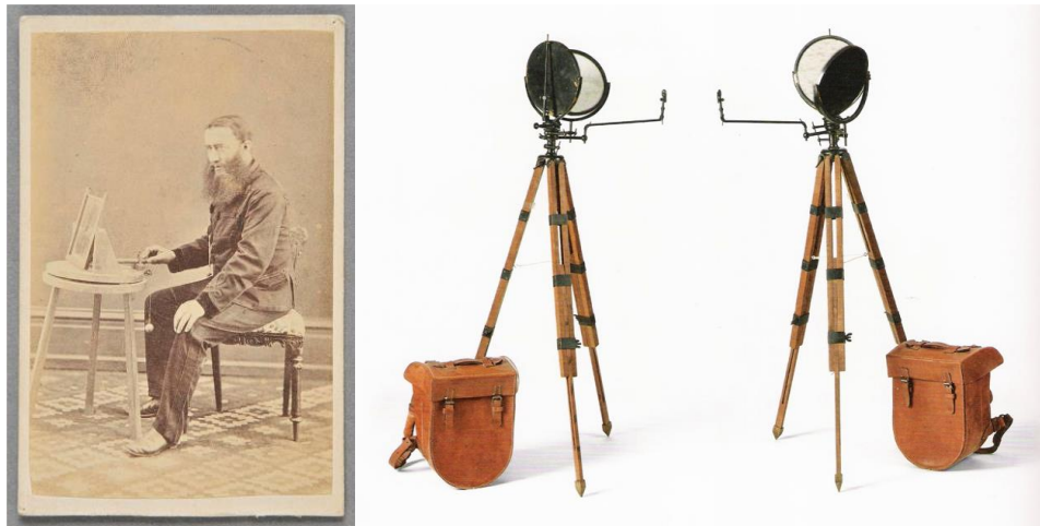
Figure 2-9 Henry Mance next to the heliograph prototype (left) [12] and two field heliographs (right) [24].
