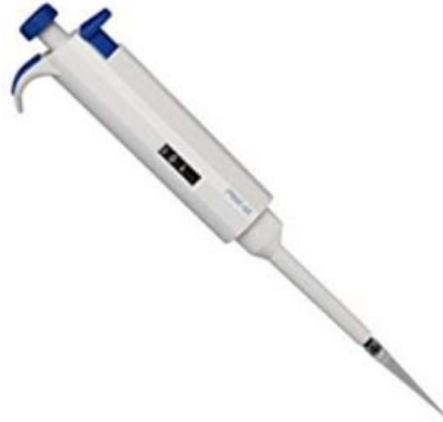
**Figura A1-0-4 Micro pipeta**
