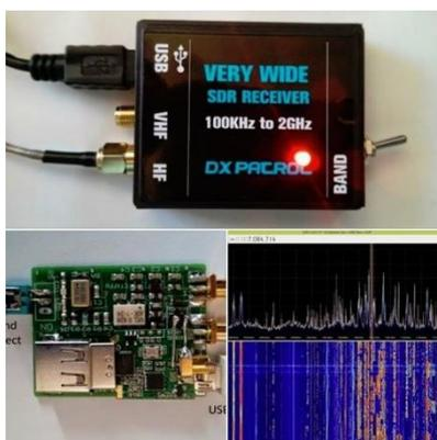
Figura 2-11 Receptor SDR DX PATROL.
