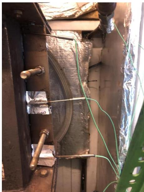
**Figura 4-7 Termopares**
