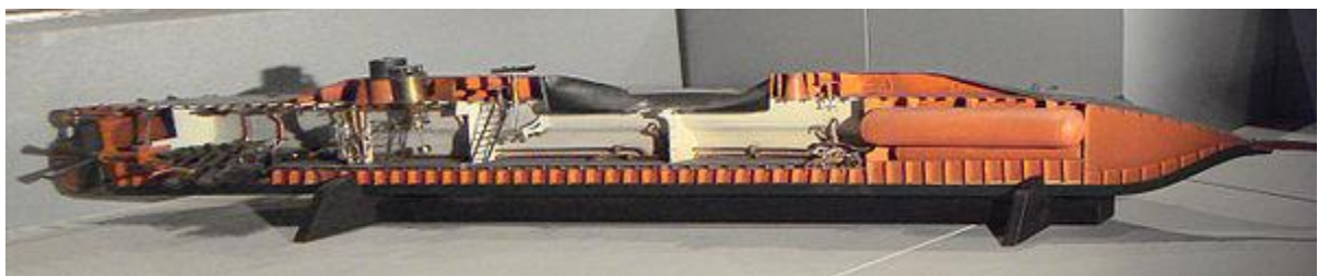
Figure 2-3. Internal view of the "Plongeur". [3]
