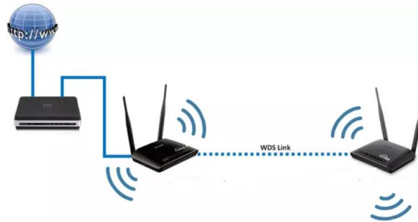
Figura 3-34 WDS (Wireless Distribution System) [79]
