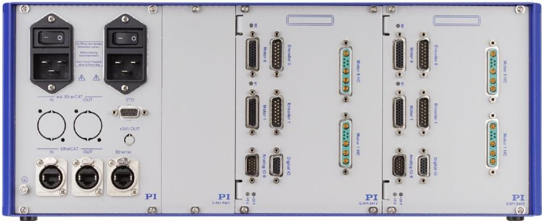
Rear panel of the G-901.R3199 with connectors
