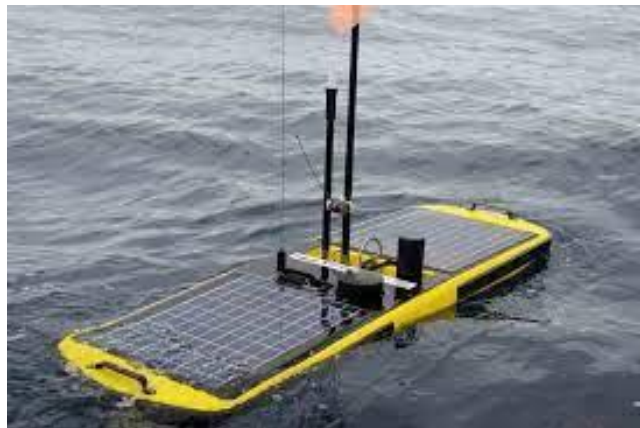
Figure 8. Wave Glider USV [40].
