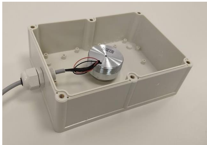
Figure 24. Vibration transducer inside the plastic box.
