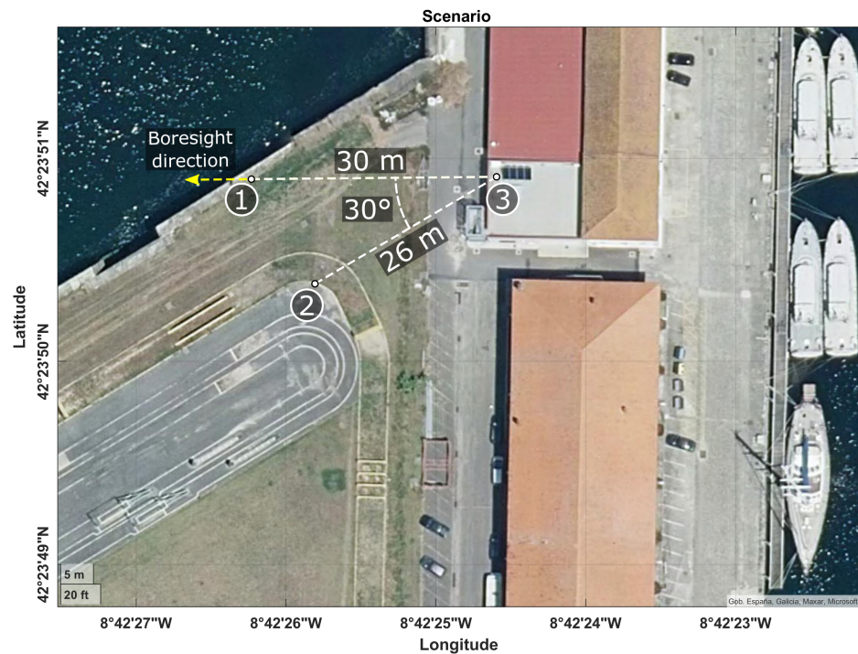
Figure 3. Scenario used in the tests: ① beacon transmitter, ② simulated source, and ③ antenna array.
