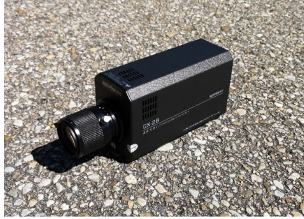
Figure 6: Measurement device used to collect luminance data.
