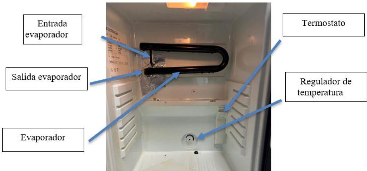
Figura 3-4 Evaporador "Electrolux"
