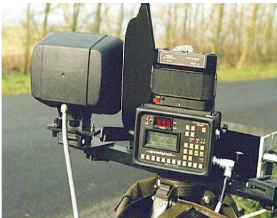
Figura 2-17. Radar Traffipax Speedophot [23].
