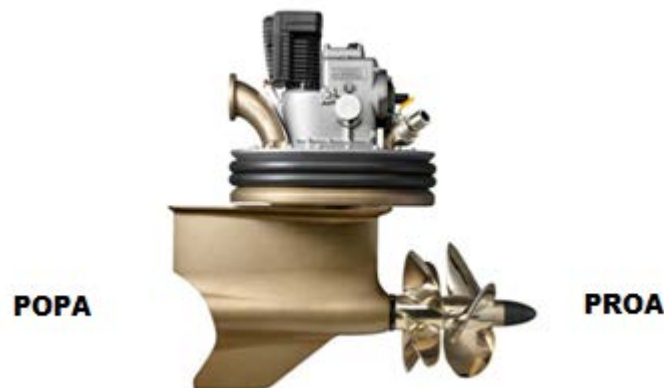
Figura 34. Volvo Penta IPS 1 Pod [35]
