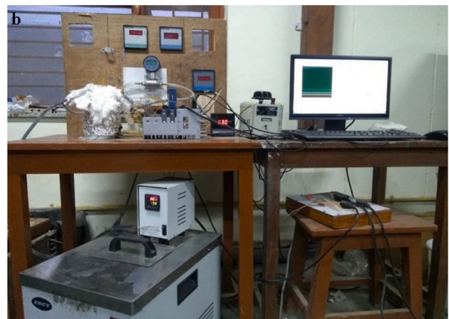
Fig. 5. Experimental setup with a minichannel device as main element: schematic diagram (a) and photograph (b) [51].
