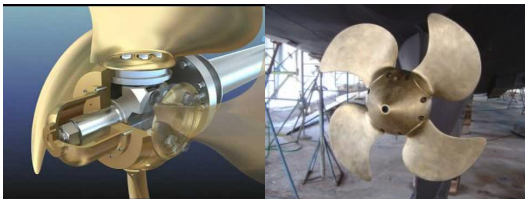
Figura 2-2 Variable Pitch Propeller. Hélices de paso variable. [6] [7]
