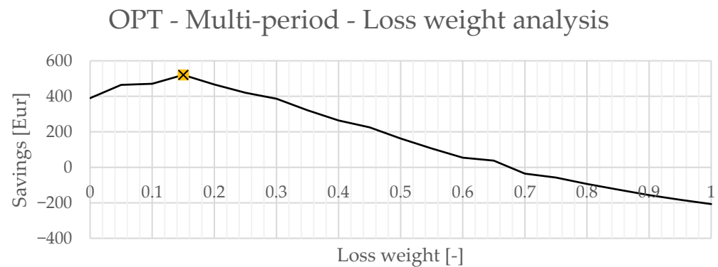
Figure 10. Results optimization for different values of battery aging cost weight ( \alpha ) in multi-period prices scenario.
