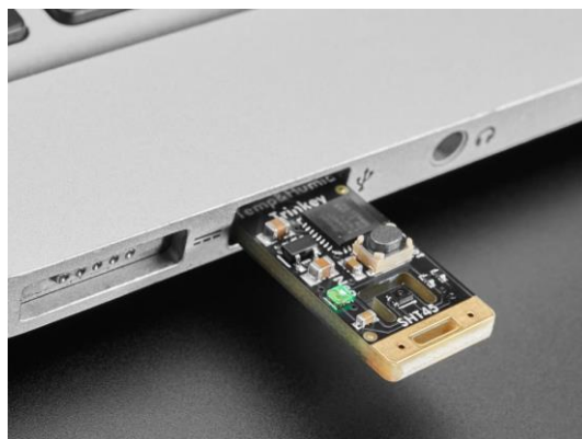
Figura 3-34 Sensor Adafruit SHT45 Trinkey [32].
