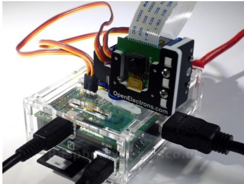
Figure 5-2 Pi Camera mounted on an electric motor with pan and tilt functionality (taken from [71])
