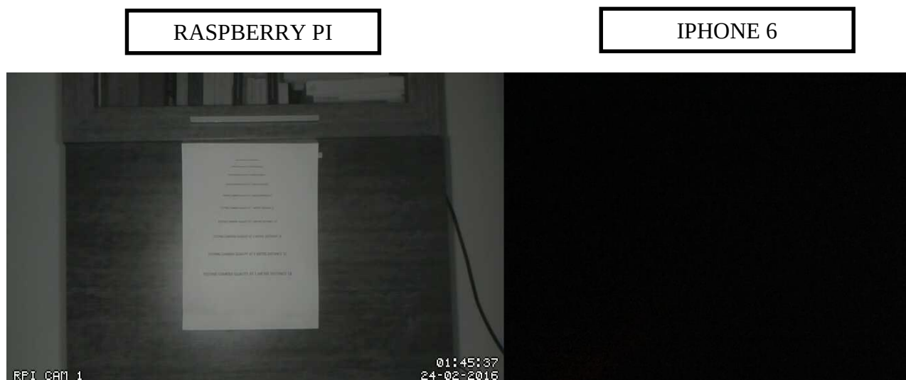
Figure 4-4 Comparison of a photo taken with no light with Pi Camera and an iPhone 6.
