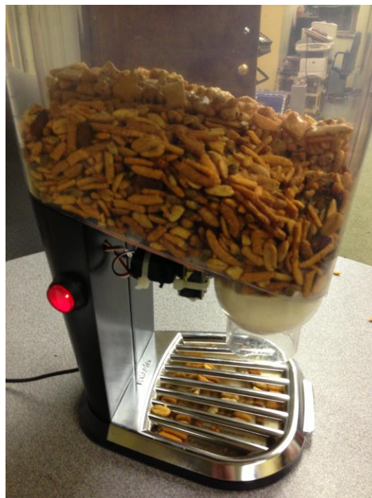
Figure 2-20 Automatic pet feeder using a Raspberry Pi (taken from [43])
