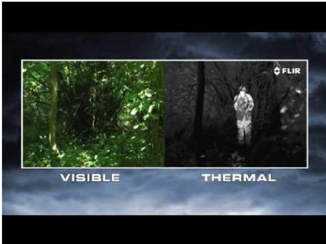
Figure 2-4 Comparison of the same scenario with visible light and thermal imaging (taken from [14])
