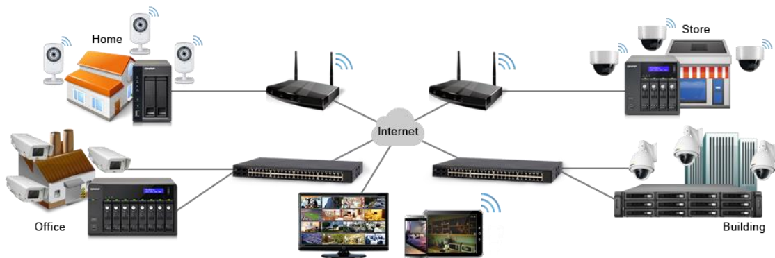
Figure 2-6 Example of how a video surveillance system with remote viewing using the Internet is configured (taken from [16])
